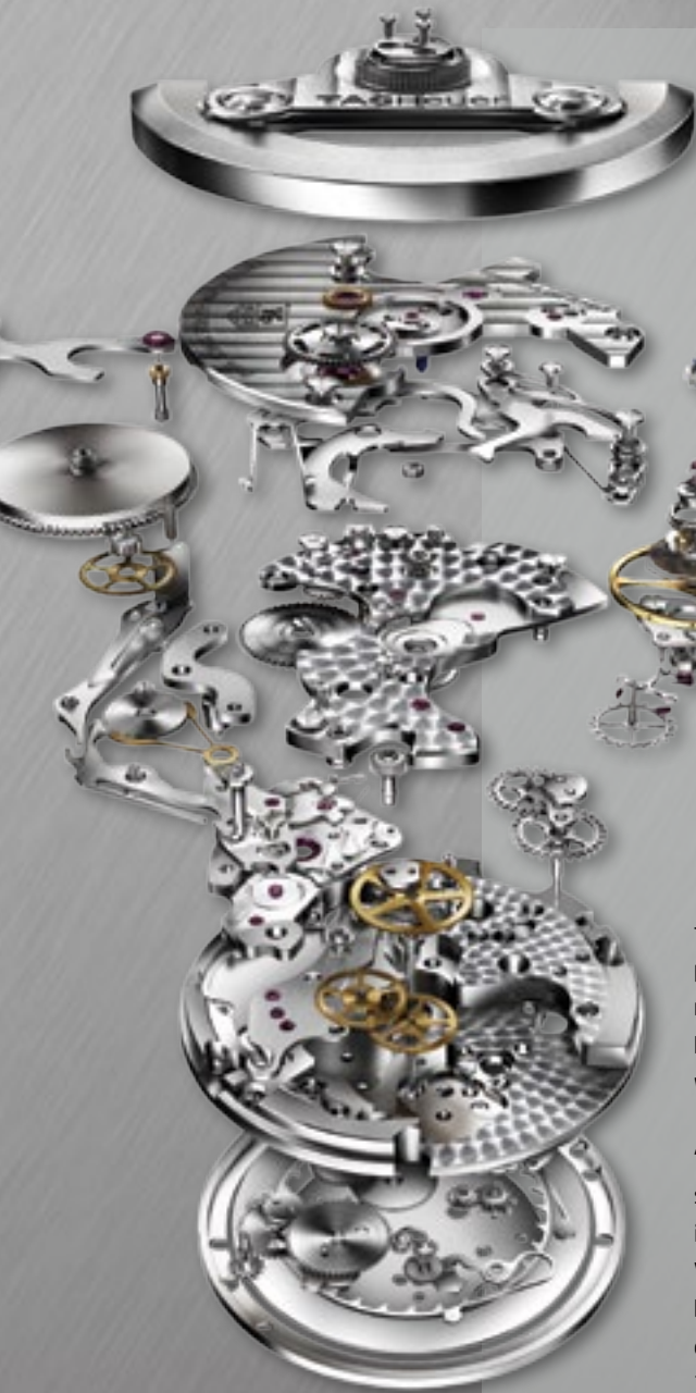
The Calibre 1887 is an integrated chronograph movement with 320 parts in total. Of that, about 270 are made in Switzerland, some by TAG Heuer/Cortech (bridges, plates, oscillating weight) and some by specialist suppliers such as Nivarox. Many of these parts have been upgraded from the original design.
