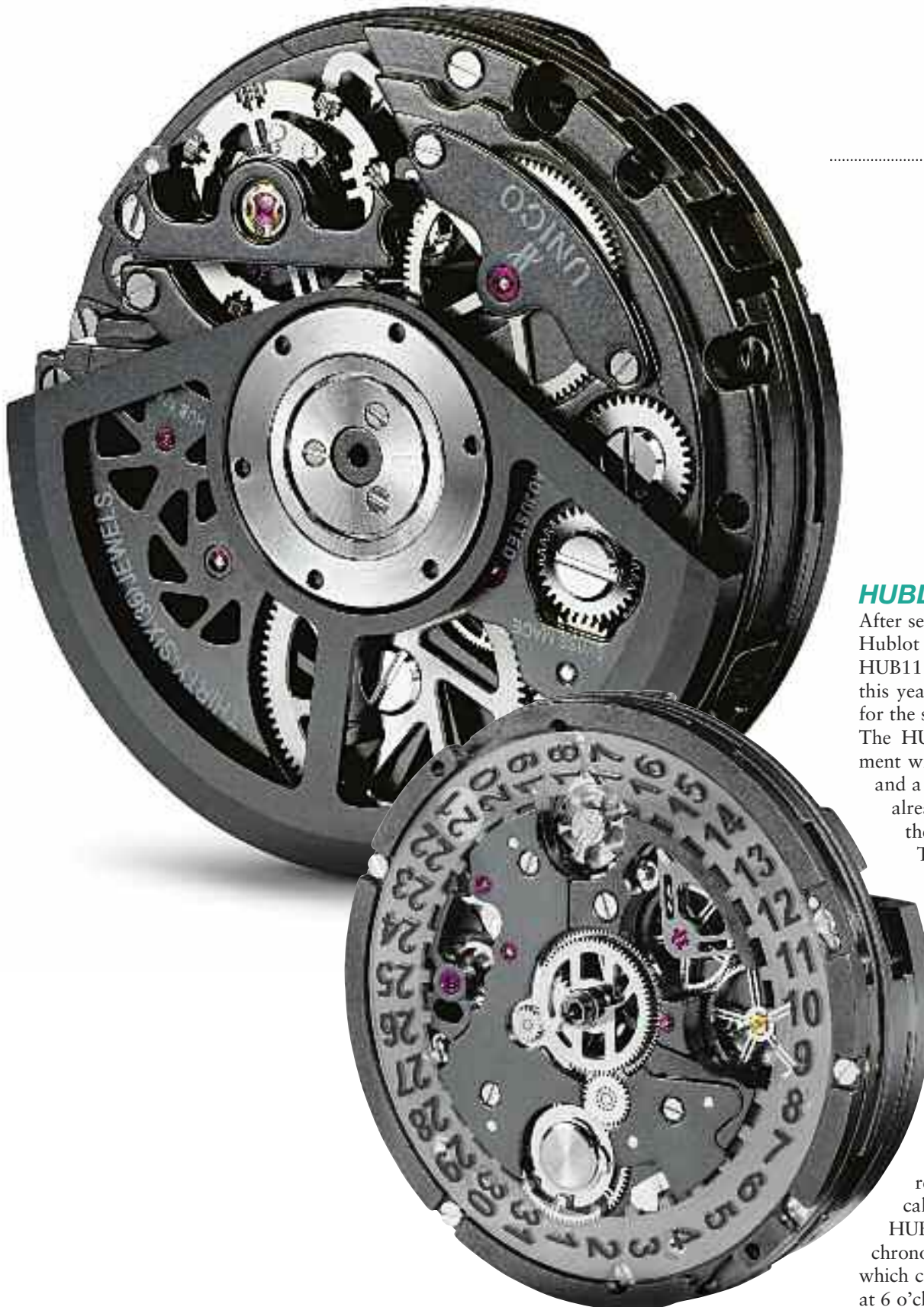
Hublot's automatic Unico movement with chronograph module
