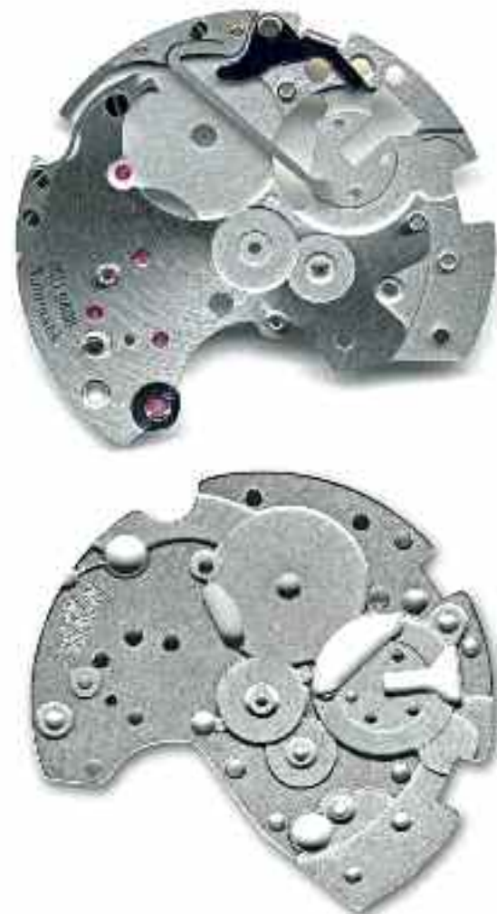
Compared to the Valjoux plate, pictured below it, Mühle's plate has an improved bearing for the crown wheel (the round milled indentation at the upper right), a Glashütte ratchet (the spring and pawl at the upper left) and a removable escape-wheel bridge (round plate at lower left)
