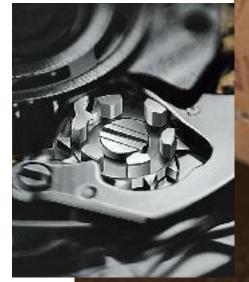
The column wheel is the heart of the chronograph. It controls all of the stopwatch functions
