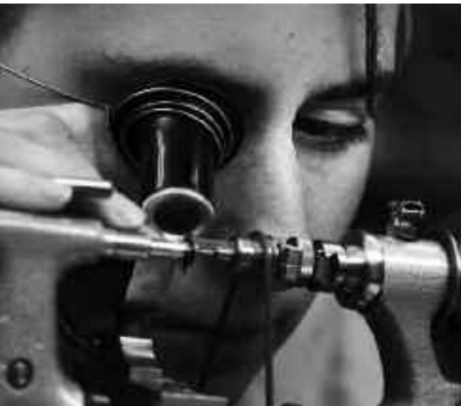
Testing watches (above) and a watchmaker performing a balance-wheel pivoting operation (left) at Manufacture Cartier
