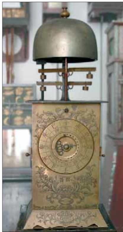
Before Japan adopted the Western time system, special clocks displayed the time according to the lunar system that was in use for several hundred years. Many, like this example in the Seiko Institute of Horology, had two verge and foliot mechanisms, instead of the single escapement used in the West.
