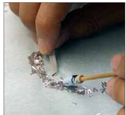
Many processes in the production of high-grade watches cannot be automated. Here, hands are examined one-by-one to eliminate any with tiny imperfections.
