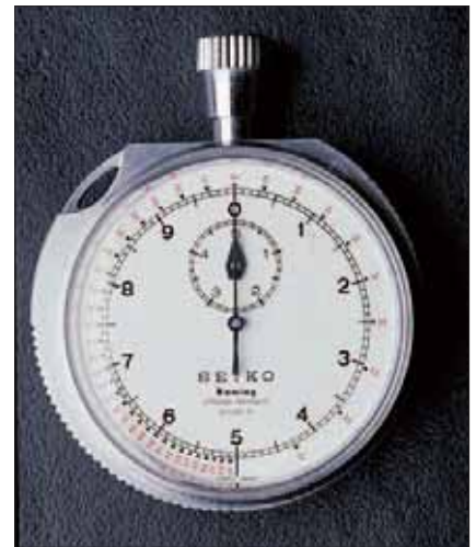
Seiko has developed special timepieces for many different sports. This example measures the number of strokes per minute in rowing competitions. It helps rowers adjust their stroke rate, but is not used for official timing.
