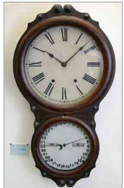
A wall clock with a second dial that shows the day, month, and date, made in the USA by Seth Thomas at the end of the 19th century.
