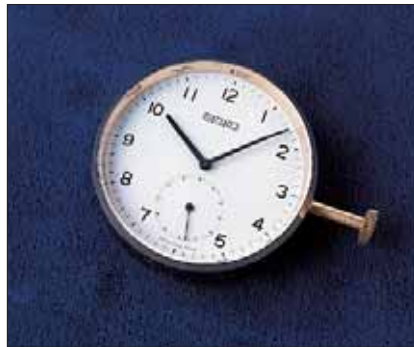
Calibre 965, was nicknamed The Potato, because of the shape of the movement inside the case. It was one of the earliest movements submitted to the Swiss competitions by the Daini Seikosha factory – it ran at 6 beats a second.
