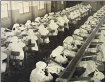
This wristwatch assembly line, around 1950, used conveyor belts to boost production and the staff wore protective clothing to protect the movements from dust.
