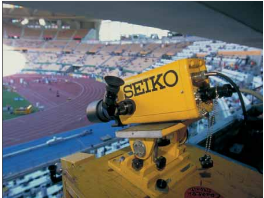
The Seiko "slit-video" photo-finish camera provides the image from which officials decide both the result and the time, to an accuracy of \frac{1}{1000} of a second.
