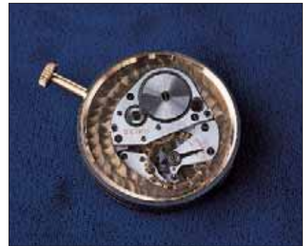
Calibre 965, was nicknamed The Potato, because of the shape of the movement inside the case. It was one of the earliest movements submitted to the Swiss competitions by the Daini Seikosha factory – it ran at 6 beats a second.
