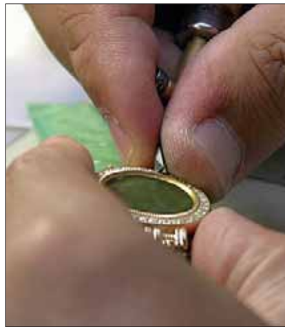
Seiko employ diamond mounters for work on their gem-set watches, as well as jewellery. Here, diamonds are set into the case of a gold watch.
