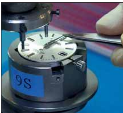
Grand Seiko movements are largely assembled by hand, so inevitably they are expensive. Here, hands are added to a watch.
