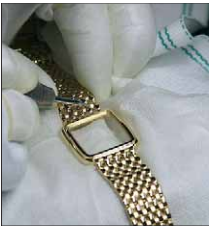
In order to produce high grade gold and jewellery models, Seiko employ craftsmen with many different skills. Goldsmiths assemble gold bracelets by hand.
