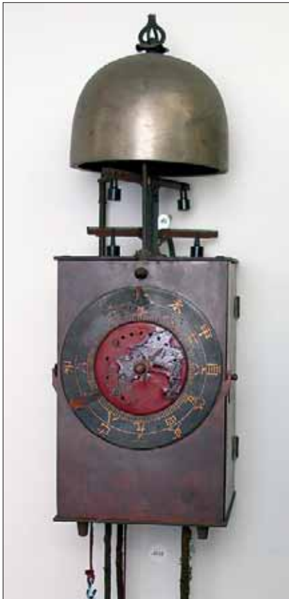
The Institute includes not only timepieces recording Seiko's own history, but also other clocks that illustrate the history of timekeeping in Japan. This is a clock with a twin verge and foliot (visible below the bell), from the era when Japan used the lunar system of timekeeping.
